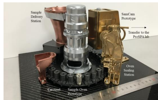
Figure 6: Solids Inlet System model including SamCam
